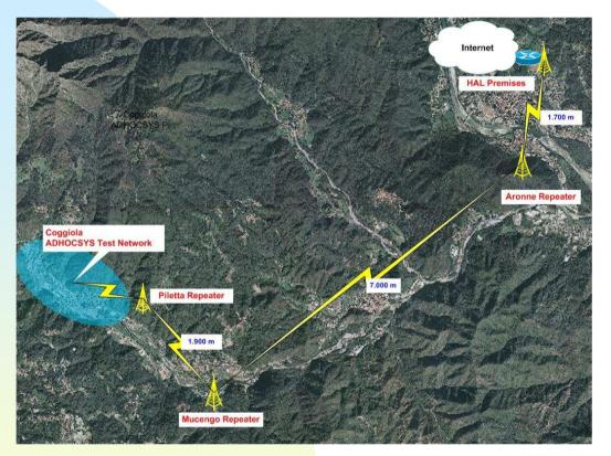
The access network consists of 10 nodes (9 static and 1 mobile), covering almost all Coggiola territory and is connected via a wireless backbone to an Internet gateway located at Hal Service's premises in Borgosesia
